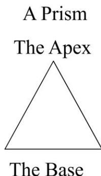
Prism is not the same as power in a lens. Power will either converge light or diverge light from a point. Prism diffracts light which is another way of saying it changes the direction of the light. If parallel light passes through a plus lens then the light would be converged to a point.
