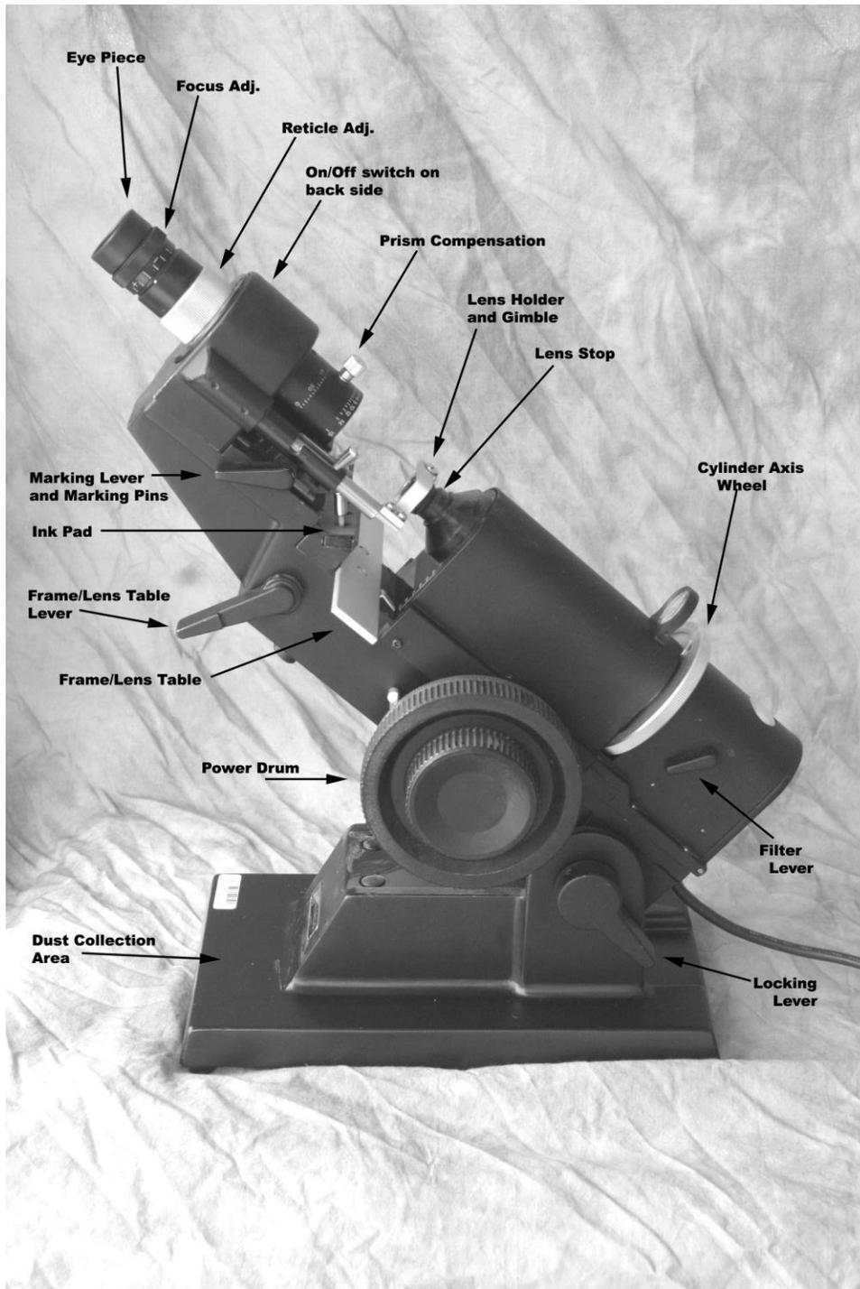
Now that you are familiar with the parts of the lensometer you should learn the basic setup of the instrument. The first thing to look at is the focus of the eyepiece. This is done by taking a white piece of paper and placing it between the prism ring and the lens stop, at an angle to shine ambient light into the instrument. Looking into the lensometer look at the reticle and make sure these lines are in focus. Change the focus with the ring on the eyepiece.
